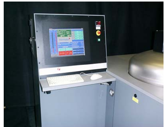
Microlink controller on vacuum furnace
