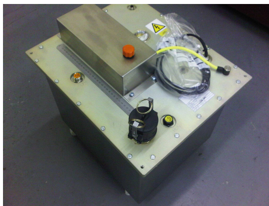
Switch mode HV system is controlled from the PLC Touch Screen control and programming in Movicon
